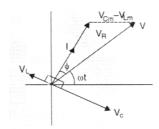
From the phasor relation, voltages  $V_L + V_R + V_C = V$ , as  $V_C$  and  $V_L$  are along the same line and in opposite directions, so they will combine in single phasor  $(V_C + V_L)$  having magnitude  $|V_{Cm} - V_{Lm}|$ . Since voltage V is shown as the hypotenuse of right-angled triangle with sides as  $V_R$  and  $(V_C + V_L)$ , so the Pythagoras Theorem results as:
