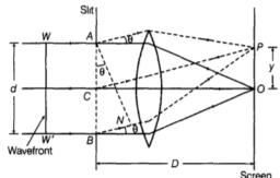
The wavelets from the single wavefront reach the centre O on the screen in same phase and hence, interfere constructively to give central maximum (bright fringe).
