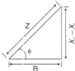
As phasor 1 is always parallel to phasor  $V_R$ , the phase angle  $\phi$  is the angle between  $V_R$  and V and can be determined from the figure.
